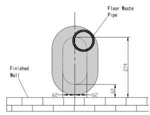
Dotted line indicates maximum offset for Waste Pipe centreline. Floor Waste Pipe must fit within shaded area.
